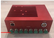
FBG interrogator (SwitchedGator)
